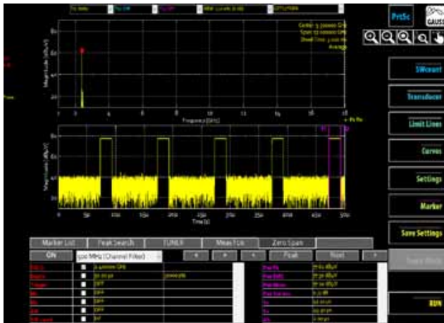
Fig. 6 – Pulse Measurement with 510 MHz Measurement Bandwidth.
